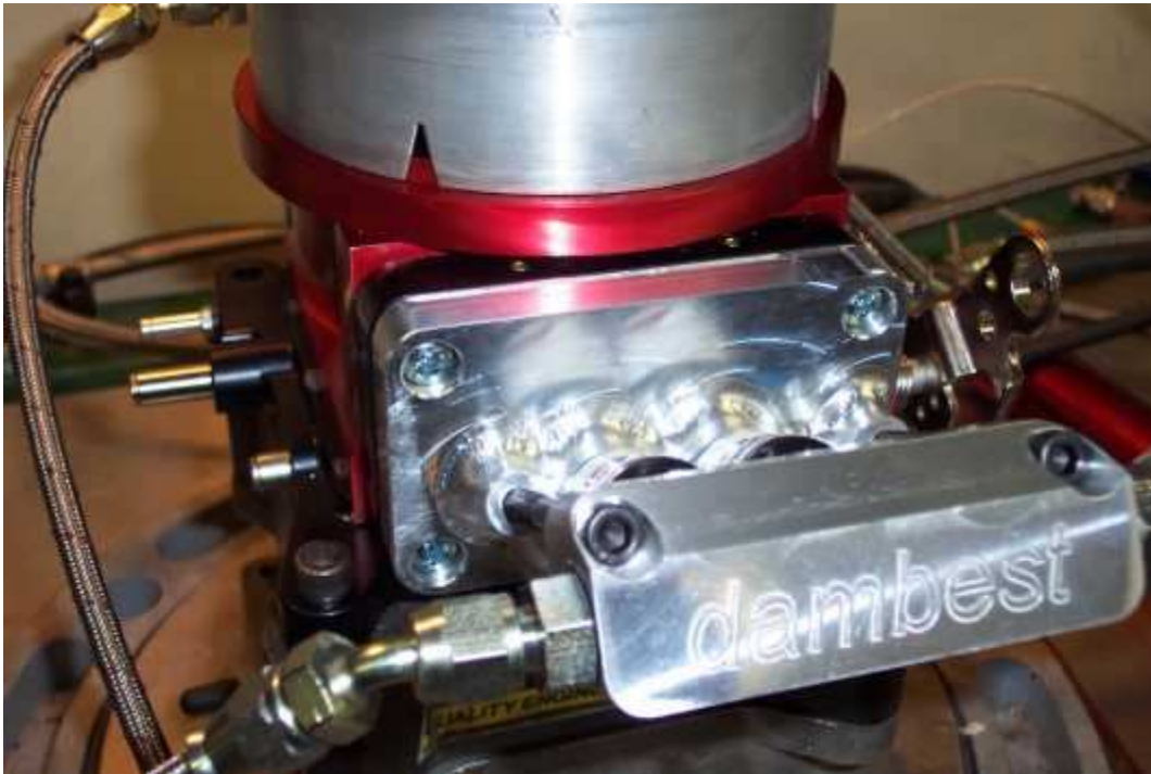
View from end: fuel rail
